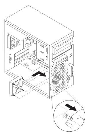
Figure 32. Installing the front fan assembly
